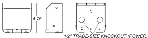
Smart-Way Raceway wall feed kit, closeup.
