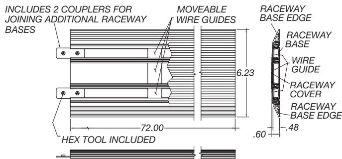
Each 6' section includes a base and cover, two couplers, moveable wire guides, raceway base edges, and a hex tool for installation. Additional Raceway lengths are available in 3-foot, 1-foot and a three part (1', 2', 3') saw-less installation kit.
