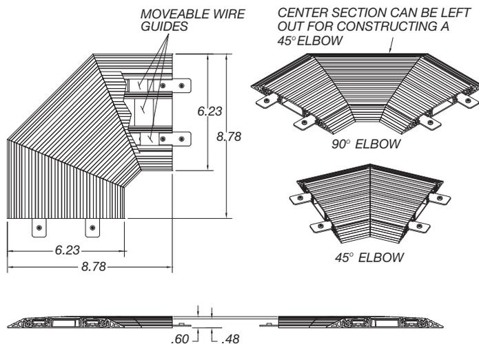
Moveable wire guides are provided with the raceway.
