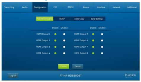
Enable/disable video resolution auto-downscaling function of HDMI output 1~8 ports.
