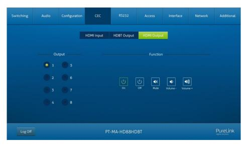
Select one or several HDMI output devices to be controlled, and then press function buttons.
