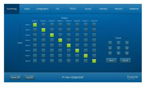
Use the 8x8 button grid on the page to set which inputs are directed to which outputs. For example, clicking the button on the Input 1 row and Output 2 column, directs input 1 to output 2.
