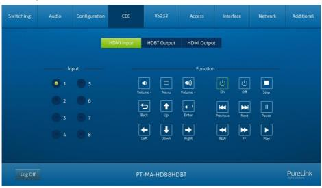
Select one or several HDMI input source devices to be controlled, and then press function buttons.
