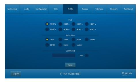
Send RS232 commands to control third-party devices which are connected to the far-end HDBaseT receivers.
