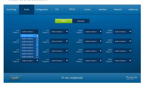
There are sixteen audio sources can be selected for eight analog L+R audio output ports, and twenty-four audio sources can be selected for four digital SPDIF output ports.
