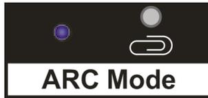
Press the button with paper clip or other sharp tool to enable the ARC mode, and then the left LED illuminates blue. Press it again to exit the ARC mode and the LED is off.
