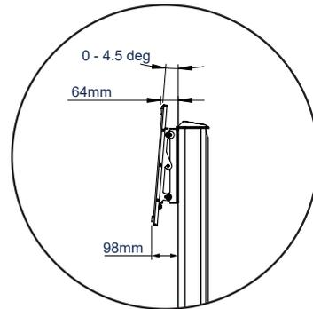
VUE DE CÔTÉ AVEC UNE INCLINAISON MAXIMALE
