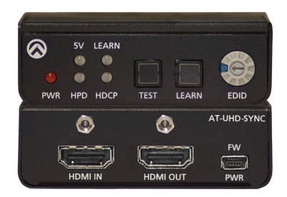
The Atlona AT-UHD-SYNC is designed to analyze errors, identify issues and restore failed HDMI signals. The UHD-SYNC's slender, palm sized design ensures easy integration into confined spaces. USB powered, with included USB power suppply or from local USB devices. With presets and learned EDID, the UHD-SYNC provides a solution whenever and wherever it is needed.
