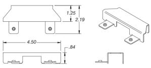
FOR USE WITH THE SMARTWAY RACEWAY.
