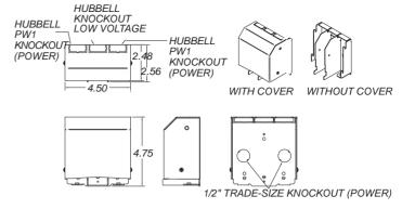
Smart-Way Raceway wall feed kit, closeup.
