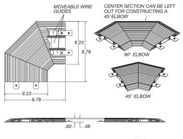
Moveable wire guides are provided with the raceway.
