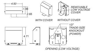
SW-WF-HP-ALM 18218 18220 SW-WF-HP-SLT SW-WF-RIN 18317 Wall Feed Rough In Box (New Construction) 18320 **SW-FCT-SLT** Raceway to Flexible Metal **Conduit Transition** 18326 SW-PKF-SFIT4 Raceway Feed from 4" Poke Through (Poke-through not included)
