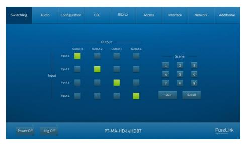
Use the 4x4 button grid on the page to set which inputs are directed to which outputs. For example, clicking the button on the Input 1 row and Output 2 column, directs input 1 to output 2.
