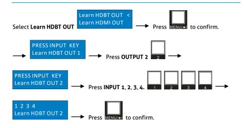
• To copy the EDID data from one HDMI output to one or several inputs:
