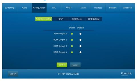
Enable/disable video resolution auto-downscaling function of HDMI output 1~4 ports.
