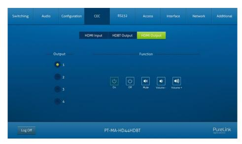
Select one or several HDMI output devices to be controlled, and then press function buttons.
