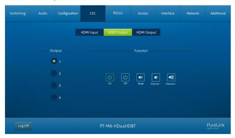
Select one or several HDBaseT output devices to be controlled, and then press function buttons.
