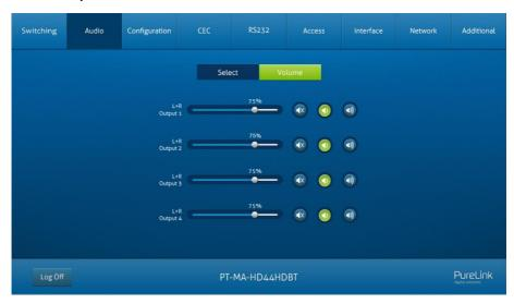
Adjust L+R output audio volume by the volume bar and the three buttons on the right side.
