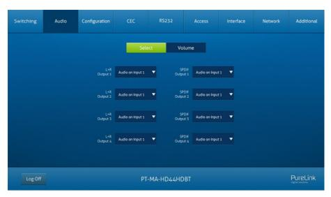
There are eight audio sources can be selected for four analog L+R audio output ports, and twelve audio sources can be selected for four digital SPDIF output ports.
