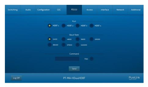
Send RS232 commands to control third-party devices which are connected to the far-end HDBaseT receivers.
