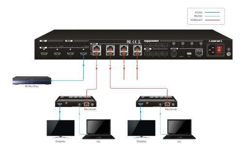
**Note:** The command "**RS232RCM**[XX]**ON.**" ([XX]=00~04) needs to be sent to enable or disable this control mode. For example, send the command "**RS232RCM00ON.**" to enable the remote-control mode for all HDBaseT outputs, and send the command "**RS232RCM00OFF.**" to disable the remote-control mode for all HDBaseT outputs. Please refer to the 8.3.1 System Control for more details.
