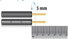
The captive screw plugs for power, audio, RS-232 and contact controls are supplied with the unit. Separate the wires about 1" (2.5 cm) long; strip off the wire insulation precisely 3/16" (5mm) from the end.
