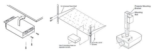
Luxi has the under desk mount sold separately (Luxi P/N 78-002-01); the product also fits many other mounting hardware from Extron, Middle Atlantic, etc. Only use the type 4-40, 3/16" (5 mm) long screws supplied with the mounting hardware to screw onto the product. Wrong
