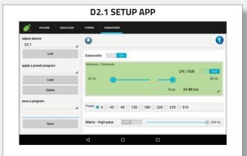
The D2.1 Setup App allows quick, visual configuration of D2.1 settings from an Android or iOS smartphone or tablet including audio-sensing for power management, source priority, EQ, subwoofer crossover, slope, phase and high-pass. Setups can be saved and modified for use in future installations.
