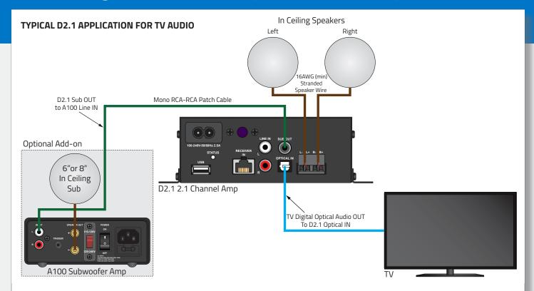
Typical System application for stereo audio and subwoofer. Amp will auto-sense TV audio (or other source) and output audio to speakers and sub amp automatically. Amp can be hidden in a cabinet and controlled via IR Repeater system using either the D2.1 IR Remote or TV Remote.
